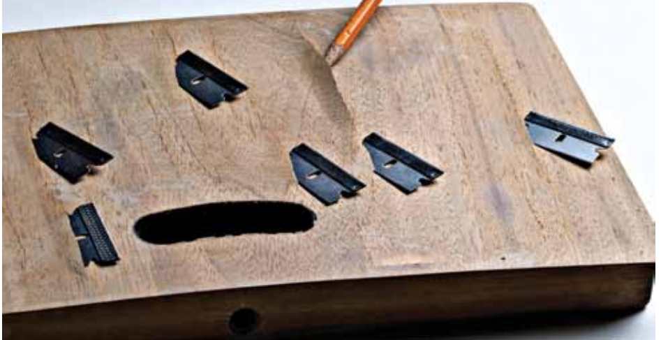
THE RAZOR BLADES AND PENCIL SHOW SOME OF THE AREAS THAT HAD POOR ADHESION BETWEEN THE SUB-VENEER AND PLYWOOD.
